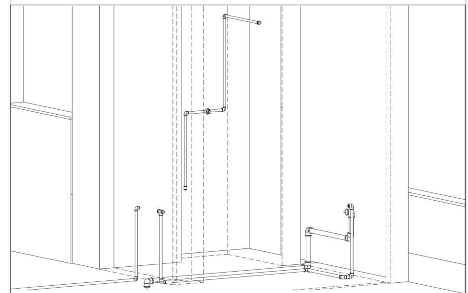
VISTA ESQUEMA HIDRÁULICO B.W.C.
